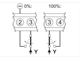
Fig. 9 Overriding the input signal Y,
