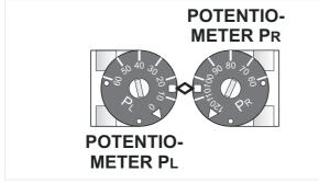
Fig. 4 Example setting of angle of rotation (PL and PR)
