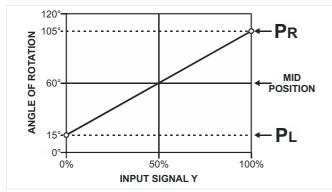
Fig. 5 Input signal Y and angle of rotation
