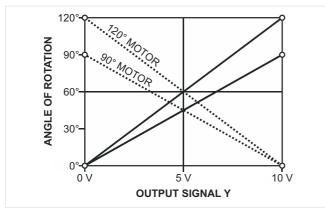
Fig. 6 Output signal Y and angle of rotation with VMU1
